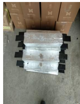
2018 - Sacrificial Aluminium Anode for Jetty Pile - PT Indah Dewi, Tarakan, Kaltara
