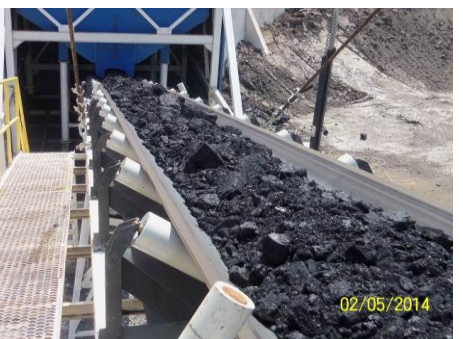
2014 - New Coal Crushing Plant Cap. 300 TPH - PT Duta Tambang Rekayasa (Medco Mining), Nunukan, Kaltara
