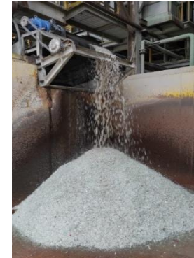
Mar 2022 - New Cullet Washing Conveyor Cap. 10 TPH - PT Kangar Consolidated Industries, Cakung, Jaktim
