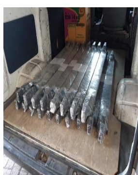
2016 s.d 2019 - Material Sacrificial Zinc Anode for CWP Discharge, Cooling Tower, Screen - PT. Cirebon Electric Power, Cirebon, Jabar
