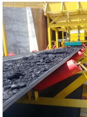
Dec 2020 - New Barge Loading Conveyor Cap. 1000 TPH – PT Borneo Emas Hitam, Loa Tebu, Kalsel
