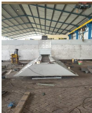
Dec 2022 - Reclaim Feeder for Coal Cap. 200 TPH - PLTU Sulut 1
