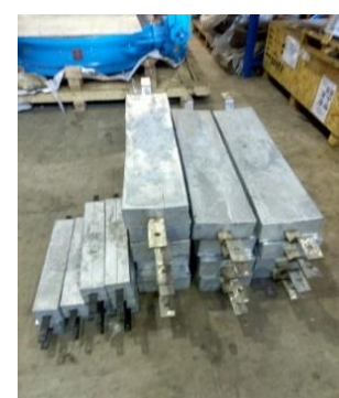
2016 s.d 2019 - Material Sacrificial Zinc Anode for CWP Discharge, Cooling Tower, Screen - PT. Cirebon Electric Power, Cirebon, Jabar
