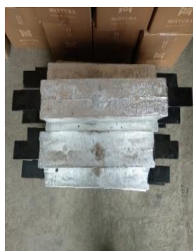
2018 - Sacrificial Aluminium Anode for Jetty Pile - PT Indah Dewi, Tarakan, Kaltara
