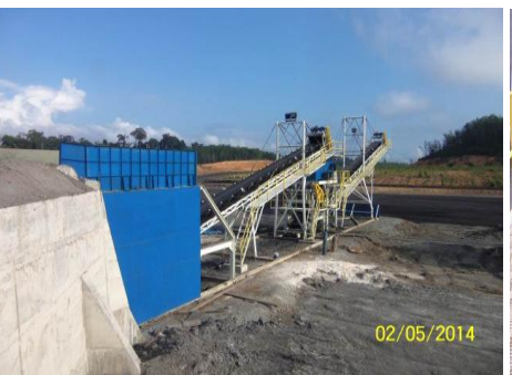
2014 - New Coal Crushing Plant Cap. 300 TPH - PT Duta Tambang Rekayasa (Medco Mining), Nunukan, Kaltara
