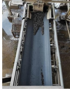
Mar 2022 - New Cullet Washing Conveyor Cap. 10 TPH - PT Kangar Consolidated Industries, Cakung, Jaktim
