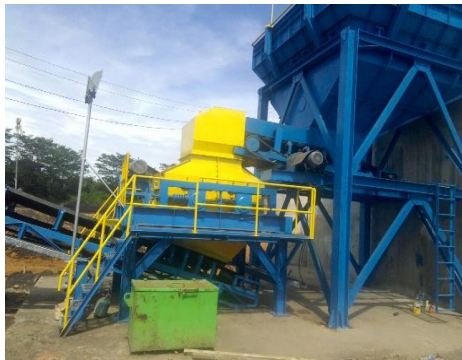
2016 - New Primary Crusher Cap. 500 TPH - PT Muara Alam Sejahtera, Lahat, Sumsel
