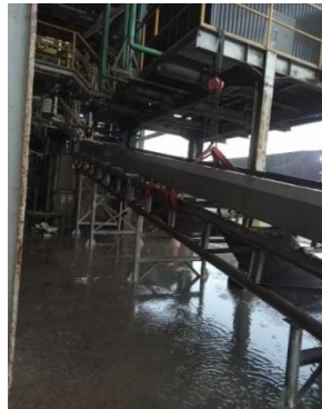
Mar 2022 - New Cullet Washing Conveyor Cap. 10 TPH - PT Kangar Consolidated Industries, Cakung, Jaktim
