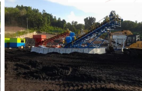
Dec 2022 – New Portable Coal Blending Plant Cap. 350 TPH - PT. Cahaya Riau Mandiri, Lahat, Sumsel
