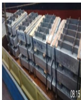
Oct 2020 - Material Sacrificial Aluminium Anode for Jembatan 2 - PT. Wassenar Karya Marga, Dompak, Tj Pinang, Kep Riau
