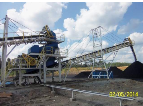
2014 - New Coal Crushing Plant Cap. 300 TPH - PT Duta Tambang Rekayasa (Medco Mining), Nunukan, Kaltara
