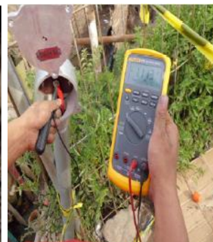
Feb 2012 - Sacrificial Magnesium Anode For Pipe Casing - PT Dover Chemical, Merak, Cilegon, Banten
