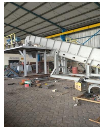
Dec 2022 - Reclaim Feeder for Coal Cap. 200 TPH - PLTU Sulut 1
