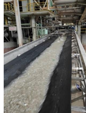
Mar 2022 - New Cullet Washing Conveyor Cap. 10 TPH - PT Kangar Consolidated Industries, Cakung, Jaktim
