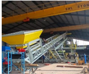
On Going - New Coal Unloading Conveyor Unit ke-2 Cap. 400 TPH - PT Siam Maspion Terminal, Gresik, Jawa Timur
